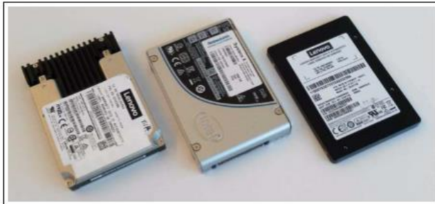
Figure 1 NVMe PCIe SSDs: (l-r): Toshiba, Intel and Samsung
